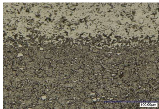
Fig. 4. Microstructure of the surface layer of P6M5K5 steel after electron beam treatment: q = 1.2 \cdot 10^4 \text{ W/cm}^2 ( V = 11 \text{ mm/s} ); x600
